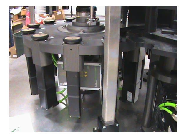
We replaced this technology completely by designing a servo motor drive for every container plate on the container table. This eliminates any limit on container shapes and label configurations and allows us to simply call up a program from the PLC for a container or package changeover.
